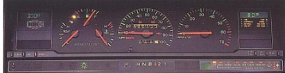
Standard full analog instrumentation includes tachometer, speedometer, odometer, trip odometer, low-fuel warning light, coolant temperature, oil pressure, fuel level gauges, and digital quartz clock. Shown with Electronic Information Package, including Trip Computer and Vehicle Maintenance Monitor (standard ES, optional LX).
