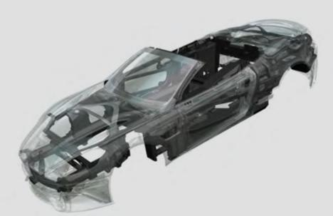
Torsional stiffness – the body structure's resistance to twisting forces – has been increased thanks to advances in alloy technology, all-carbon body panels, a new front suspension strut and body brace.
