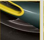
Carbon-Fibre front splitter
