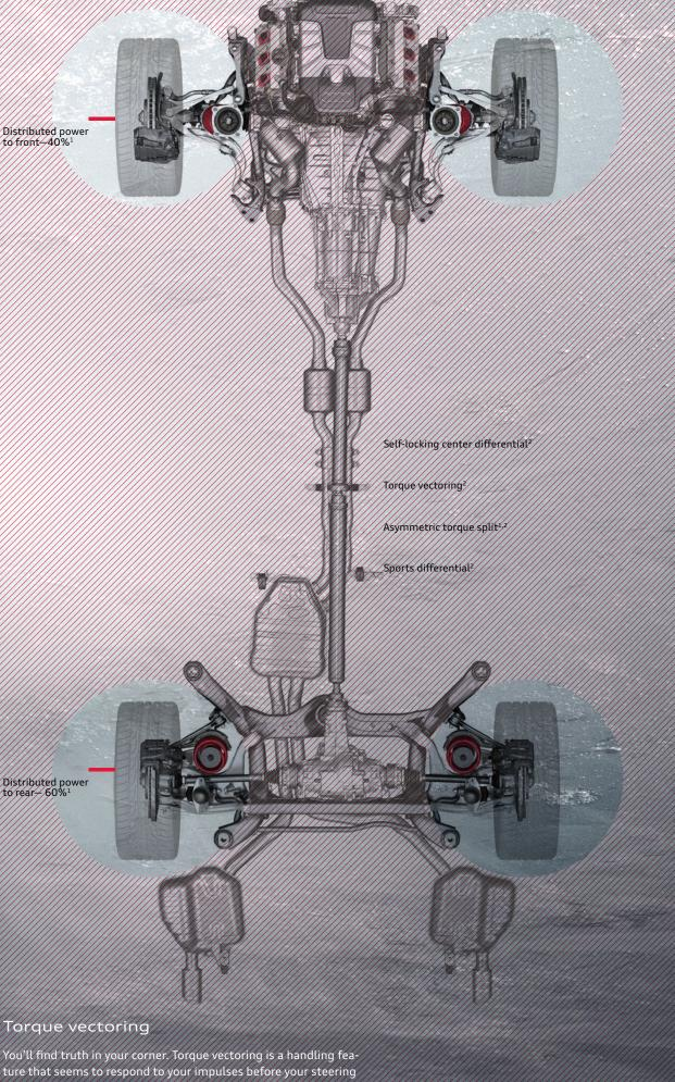
You'll find truth in your corner. Torque vectoring is a handling feature that seems to respond to your impulses before your steering input. An evolution of cross-axle lock, this system works within the Audi quattro® all-wheel drive system while utilizing Electronic Stability Control (ESC) and the Anti-lock Braking System (ABS) to help sense reduced load or wheel-spin on the inner cornering tire, making turns smoother and more responsive.<sup>2</sup>
