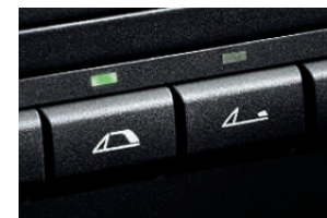
■ Power softtop roof control switch for fully automatic opening and closing of the roof is within arm's reach of the driver and front passenger. Softtop will open and close while traveling at speeds of up to 25 mph.
