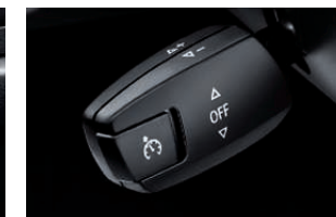
■ Cruise Control lets you store and keep to a chosen speed above 20 mph. It is activated via the left-hand steering column switch and deactivated by applying the brakes or via the switch. (Cruise Control is not a substitute for the driver's own responsibility in adjusting speed and otherwise controlling the vehicle. Due to road, traffic and visibility conditions, the driver decides whether and how the system is used.)
