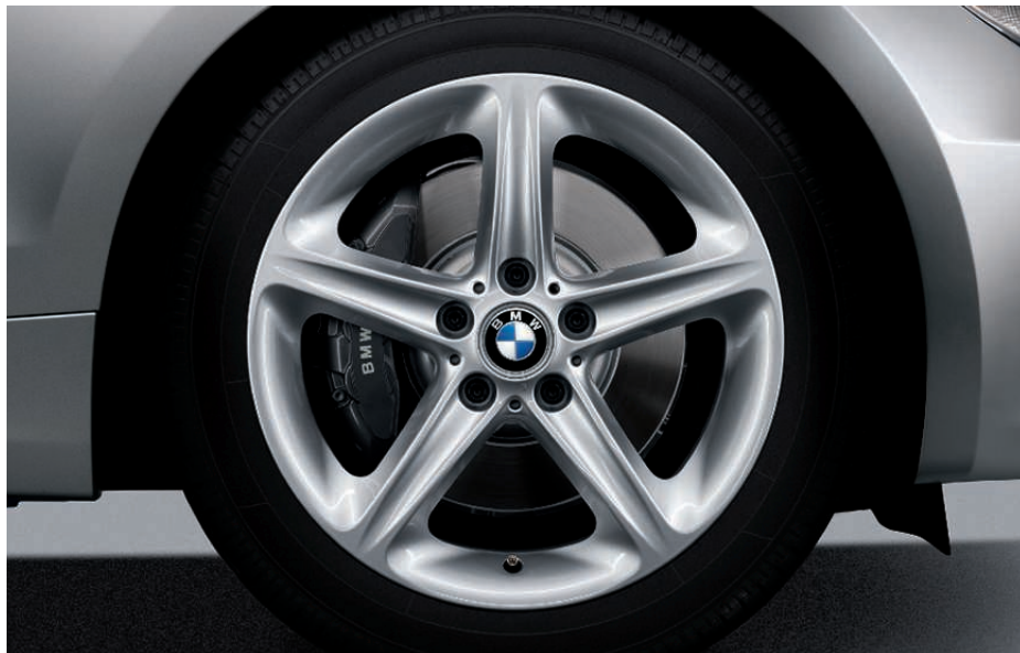
□ Star Spoke (Style 264) light alloy wheels and run-flat 1 performance tires. 2 In front: 18 x 7.5 wheels and 215/40 tires; in back: 18 x 8.5 wheels and 245/35 tires. 3 (Included in 135i Sport Package.)
