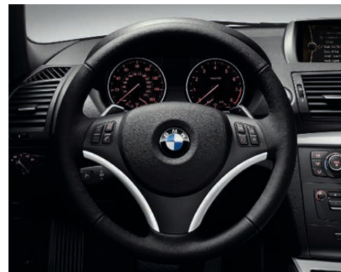
■ Three-spoke leather-wrapped multi-function sport steering wheel lets you keep both hands on the wheel while adjusting various comfort functions, such as controls for audio system, cruise control and hands-free phone controls.
