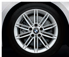
Double Spoke (Style 207M) light alloy wheels and run-flat 1 performance tires. 2 In front: 17 x 7.0 wheels and 205/50 tires; in back: 17 x 7.5 wheels and 225/45 tires.
