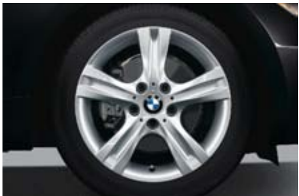
Equipped with the Sport Package, the 128i Coupe shows off its star power with attractive Star Spoke (Style 262) light alloy wheels. In front: 17 x 7.0 wheels and 205/50 run-flat 1 performance tires; at the rear: 17 x 7.5 wheels and 225/45 run-flat 1 performance tires. 2
