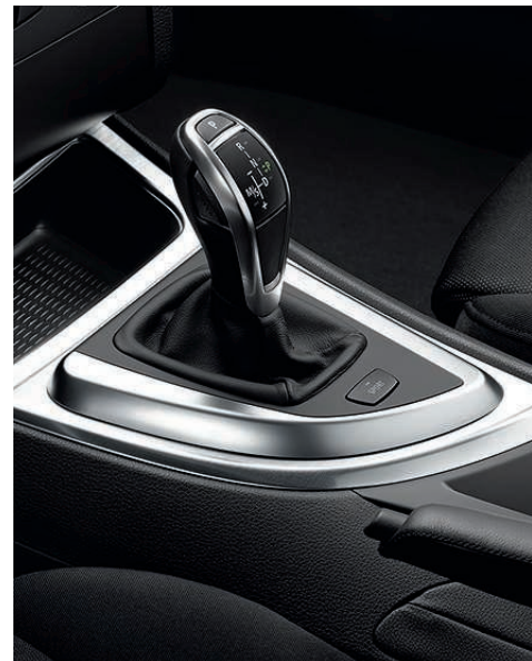
7-speed Double Clutch Transmission (DCT) in the 135i and 135is achieves smooth, lightning-quick gear changes by automatically shifting between two transmission structures: while one gear is disengaging, the next is already in position. The result is quicker acceleration and enhanced fuel efficiency. You can also shift gears manually via steering wheel-mounted paddle shifters or by moving the gear selector lever forward/rearward.
