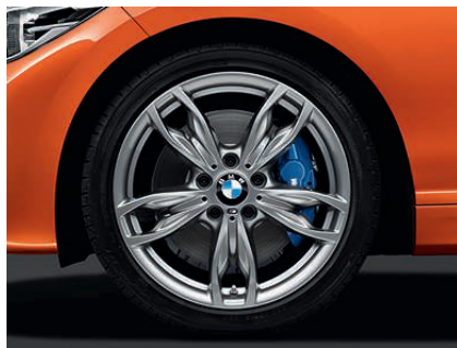
18" M light alloy wheels Double-spoke style 436 M with mixed tyres, front 7.5 J x 18 with 225/40 R 18 tyres, rear 8 J x 18 with 245/35 R 18 tyres.
