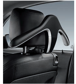
Travel & Comfort system Coat Hanger ensures crease-free transport of clothing. A retractable hook allows this item to also be used away from the car.
