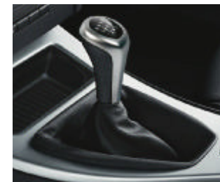
■ 6-speed manual transmission delivers a precise, athletic feel. Its responsiveness is due, in part, to the enhanced synchronization of shifts from neutral to each gear. A shortened shift lever and "throw" add to the sporty feel of the gearbox. The sixth gear drops revs at highway speeds for smooth cruising.
