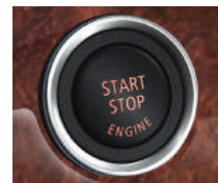
■ Engine Start/Stop button 4 and remote key control the engine. Upon inserting the remote key into the starter switch slot, and the electronic identification system confirming that it is the correct remote key, the engine can be started (or later, shut off) by pressing the Start/Stop button.
