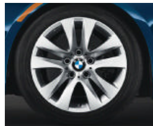
■ V Spoke (Style 338) 17 x 8.0 light alloy wheels with 225/45 run-flat 1 all-season tires. 3 (Standard on 328i.)
