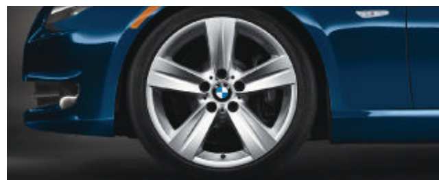
□ Star Spoke (Style 189) light alloy wheels with run-flat 1 performance tires. 2 In front: 18 x 8.0 wheels with 225/40 tires; in back: 18 x 8.5 wheels with 255/35 tires. 3 (Included in 328i Sport Package.)
