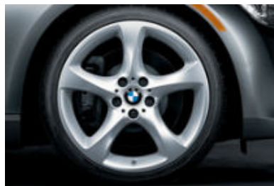
Star Spoke (Style 230) light alloy wheels and run-flat 2 performance tires. 3 In front: 19 x 8.0 wheels and 225/35 tires; in back: 19 x 9.0 wheels and 255/30 tires. (opt. on 335i, requires optional Sport Package)
