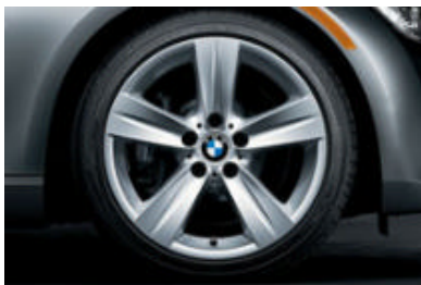
Star Spoke (Style 189) light alloy wheels and run-flat 2 performance tires. 3 In front: 18 x 8.0 wheels and 225/40 tires; in back: 18 x 8.5 wheels and 255/35 tires. (335i Sport Package; opt. on 335xi, requires optional Sport Package)
