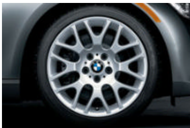
Cross Spoke (Style 197) light alloy wheels and run-flat 2 performance tires. 3 In front: 18 x 8.0 wheels and 225/40 tires; in back: 18 x 8.5 wheels and 255/35 tires. (328i Sport Package; opt. on 328xi, requires optional Sport Package)
