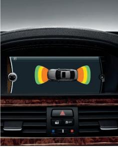
Park Distance Control uses ultrasonic sensors in the front and rear bumpers to help you judge the distance to other vehicles and unseen objects when parking. While engaged in a parking maneuver, the image on the screen visually changes and warning beeps come faster as your bumper approaches a stationary object, turning into a constant tone when the distance is less than 12 inches.
