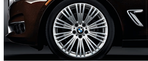
W Spoke (Style 440) 19 x 8.0 front, 19 x 9.0 rear light alloy wheels and 225/45 front, 255/40 rear summer tires . 2,3 (Includes increased top-speed limiter.)
