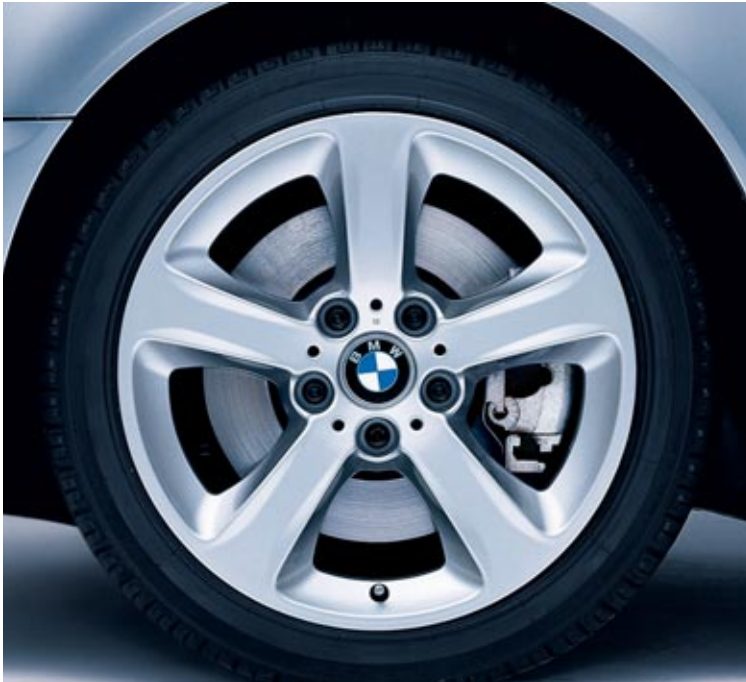
17 x 70 Star Spoke (Styling 137) alloy wheels and 205/50R-17 all-season tires on the 330i and 330xi Sedans provide reassuring performance in dry and wet weather. (incl. in 325xi Sport Package)
