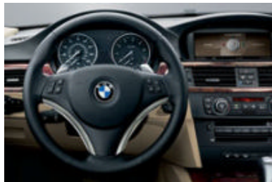
Three-spoke, leather-wrapped multi-function sport steering wheel lets you keep both hands on the wheel while adjusting various comfort functions, such as changing the radio, CD selections and volume. Optional Voice Command (included with optional Navigation system) can be used to change radio stations and audio selection, Navigation system destinations, and (accessory) telephone entries. (shown with optional paddle shifters)
