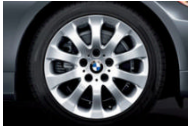
17 x 8.0 Star Spoke (Style 159) light alloy wheels with 225/45 run-flat 6 all-season tires. (included in 328xi Sport Package)
