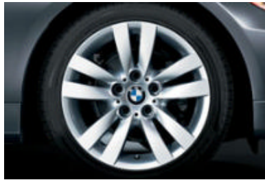
Double Spoke (Style 161) light alloy wheels and run-flat 6 performance tires. 7 In front: 17 x 8.0 wheels and 225/45 tires; in back: 17 x 8.5 wheels and 255/40 tires. 8 (included in 328i Sport Package; opt. in 328xi, requires optional Sport Package)
