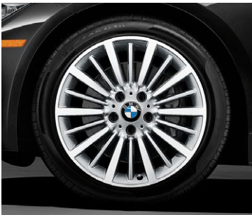
Multi Spoke light alloy wheels (Style 416) with 18 x 8.0 and 225/45 run-flat 1 all-season tires 2 .
