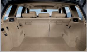
Lowering the 60/40 split-folding rear seats increases cargo space, as does a hidden storage compartment underneath the cargo floor. A handy power socket adds to the practicality. The rear cargo area provides 24.8 cu. ft. of storage with the rear seats in the upright position. With the rear seats folded down, the cargo area can be expanded to an impressive 58.0 cu. ft.
