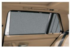
☐ Manual roller sunblind for rear side windows help keep the sun's heat and glare out of the passenger compartment while providing privacy for rear-seat passengers. Helps keep the sun's heat and glare out of the passenger compartment, and creates a comfortable environment for sleeping infants and children.
