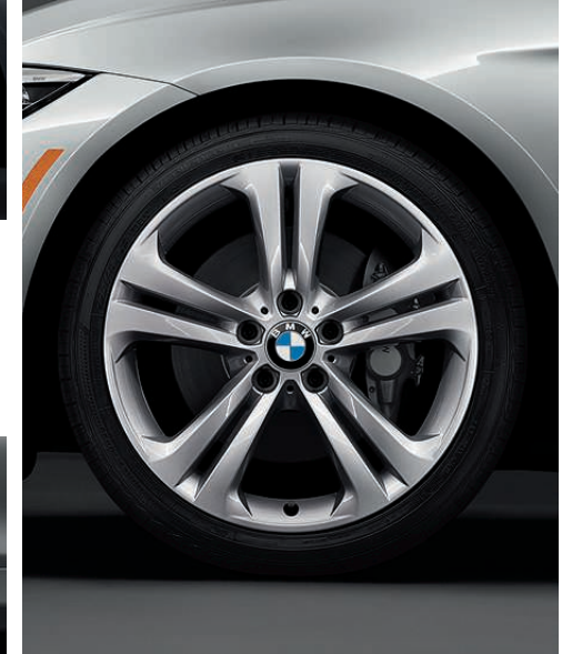
Double Spoke (Style 401) 4 19 x 8.0 front, 19 x 8.5 rear light alloy wheels and 225/40 front, 255/35 rear run-flat 1 performance tires . 2,3 (Requires M Sport brakes; includes increased top-speed limiter.)
