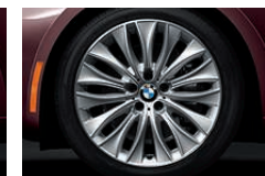
Multi Spoke (Style 459) 20 x 8.5 front, 20 x 10.0 rear light alloy wheels and 245/40 front, 275/35 rear run-flat 1 performance tires. 2,3
