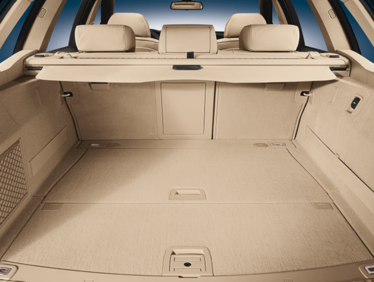
The cargo area cover tilts up whenever the tailgate or rear window is opened.
