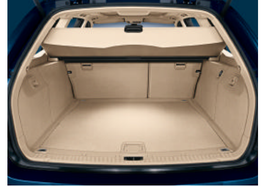
The cargo area cover tilts up whenever the tailgate or rear window is opened.
