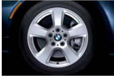
■ 17 x 7.5 Star Spoke (Style 243) cast alloy wheels with 225/50R-17 all-season tires. (std. on 535i/535xi)
