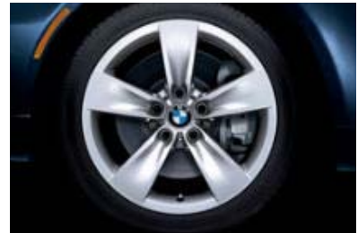
18 x 8.0 Star Spoke (Style 246) cast alloy wheels with 245/40R-18 run-flat performance tires. 3 (528i Sport Package; optional in 528xi with Sport Package; spare is a space-saver wheel and tire)
