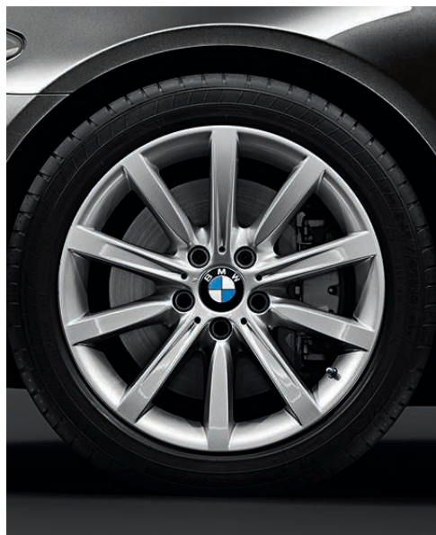
Star Spoke (Style 365) 18 x 8.0 light alloy wheels and 245/45 run-flat 1 all-season tires. 2
