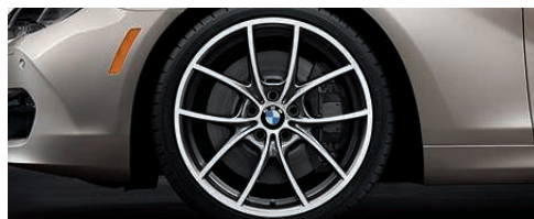
V Spoke (Style 356) 20 x 8.5 front, 20 x 9.0 rear light alloy wheels with 245/35 front and 275/30 rear run-flat 1 performance tires 2,3 .
