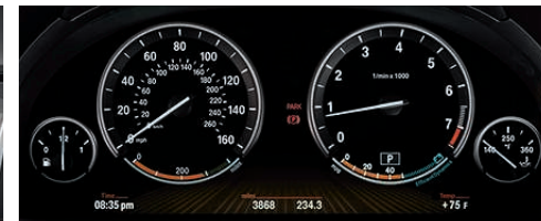
Instrument cluster displays speedometer, tachometer, fuel gauge and engine oil temperature. Below the four dials is a high-resolution Info Display that shows data such as current fuel consumption, range, on-board computer functions, mileage and trip information.
