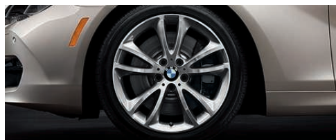
V Spoke (Style 366) 19 x 8.5 front, 19 x 9.0 rear light alloy wheels with 245/40 front and 275/35 rear run-flat 1 performance tires 2,3 .
