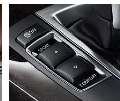
Driving Dynamics Control adjusts driving characteristics by pressing a button to select one of five settings. Choosing COMFORT, NORMAL, SPORT, SPORT+ or ECO PRO mode adjusts the engine-throttle response, shift characteristics and power-steering assist. Another button disengages the traction control feature when driving on sand, gravel, or deep or packed snow.
