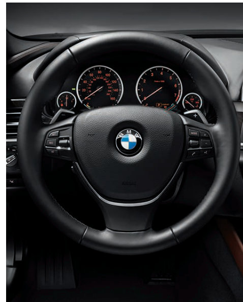
Three-spoke leather-wrapped multi-function sport steering wheel , featuring power tilt/telescoping adjustments, lets you keep both hands on the steering wheel while adjusting the audio, as well as your BMW-tested, Bluetooth ® enabled mobile phone.* The left-hand buttons operate all Cruise Control functions, while those on the right control audio functions, such as the radio, your mobile phone and Voice command.
