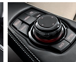
Ceramic controls present a deep black glazed finish to various controls, such as the iDrive Controller bezel, front and rear ventilation controls, and audio controls. The black ceramic provides a rich, custom look and unusually unique feel to the interior.
