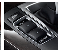
Driving Dynamics Control adjusts driving characteristics by pressing a button to select one of five settings. Choose COMFORT, COMFORT+, SPORT, SPORT+ or ECO PRO mode to adjust the engine-throttle response, shift characteristics and power-steering assist. Another button disengages the traction control feature when driving on sand, gravel, or deep or packed snow.
