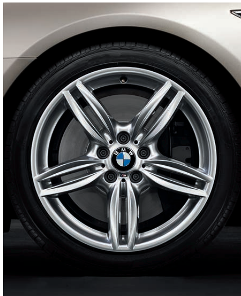
Double Spoke (Style 351M) light alloy wheels. With run-flat 1 performance tires 2, 3 : 19 x 8.5 front, 19 x 9.0 rear and 245/40 front, 275/35 rear tires. (Includes increased top-speed limiter.) With run-flat 1 all-season tires 2 : 19 x 8.5 wheels and 245/40 tires.
