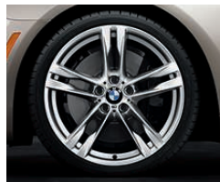
Double Spoke (Style 373M) 20 x 8.5 front, 20 x 9.0 rear light alloy wheels with 245/35 front and 275/30 rear run-flat 1 performance tires 2, 3 . (Includes increased top-speed limiter.)
