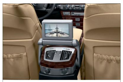
The **rear-seat monitor**, mounted on a folding arm on the rear center console, is a 6.5-inch, 16:9 aspect color screen with a resolution of 400 x 240 pixels. An integrated photocell constantly adjusts brightness for good visibility at all times.
