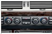
■ Automatic front climate control, adjusted through dash-mounted dials or the iDrive system, keeps the 7 Series cabin comfortable by adjusting left/right and front/rear temperature settings, air-flow volume and distribution, automatic recirculation control, heat at rest, adjustable air outlets in the B pillars, and more.
