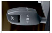
■ Programmable cruise control can be pre-programmed with up to six cruising speeds. It can retrieve them at any time by pushing the stalk forward or pulling it back. Pre-programmed speeds appear as arrows along the speedometer scale.
