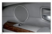
■ Standard audio system generates powerful sound through 10 speakers, including midrange speakers in each front door and each side of rear hat-shelf; tweeters in the front door mirror triangles; and subwoofers under the front seats. (750i/750Li)
