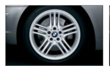
■ 19" Star Spoke (Style 89) cast alloy wheels and performance tires.¹ Front: 19 x 9.0 wheels, 245/45R-19 tires; rear: 19 x 10.0 wheels, 275/40R-19 tires. (std. on 760Li; not available on 750i/750Li)
