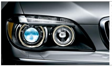
■ Xenon Adaptive Headlights illuminate the road ahead and to the side with brilliant clarity; Xenon low- and high-beam headlights also have an auto-leveling feature. BMW Adaptive Headlights illuminate the road around corners by directing the headlights into and through the bend, as soon as the vehicle begins cornering.
