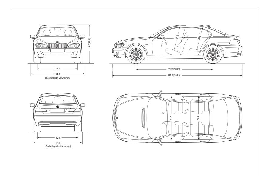
All dimensions shown in inches. Figures in [ ] apply to the 750Li/760Li; all other figures apply to 750i. Wheels shown in technical drawing are not available in the U.S.
