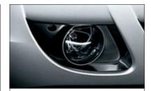
■ Halogen foglights are cleanly integrated in the front air dam. Ellipsoid free-form technology ensures an even spread of light onto the road for extra safety in bad weather and poor visibility.
