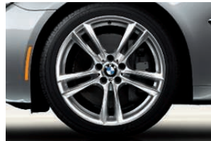
Double Spoke (Style 303M) M light alloy wheels, 20x8.5 front, 20x10.0 rear, with 245/40 front, 275/35 rear run-flat performance tires . 1
