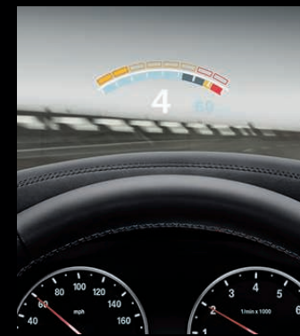
The M-specific BMW Head-up Display projects all relevant driving data – and, if requested, Speed Limit Info – directly onto the windshield.
