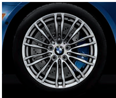
Double Spoke forged light alloy wheels (Style 345M) , 19 x 9.0 front, 19 x 10.0 rear; and 265/40 front, 295/30 rear performance tires . 1
