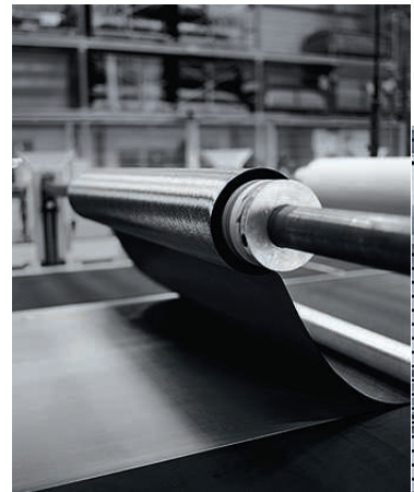
Carbon sheets are delivered on rollers and layered one atop the other (right). Robots transport the pre-formed roof (far right) to the large press for injection of the resin (below).
