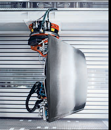
A CARBON FIBER ROOF, AT ABOUT HALF THE WEIGHT OF STEEL, LOWERS THE CENTER OF GRAVITY TO ENHANCE DYNAMICS.
