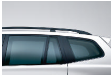
Privacy glass in the rear and rear side windows enhances passenger privacy, while reducing sun glare and interior heat.
