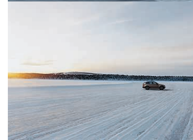
The low frictional coefficients on the frozen lakes are perfect for repeatable test drives at the limits of adhesion.
