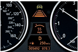
Active Cruise Control (ACC) with Stop & Go lets you preset desired speed and following distance. When ACC recognizes slower vehicles ahead, it reduces your speed to maintain the preset distance. Stop & Go can bring you to a complete stop if traffic calls for it. When you press the accelerator, ACC resumes speed according to your presets.
