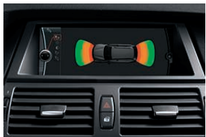
Park Distance Control uses eight sensors – four in the front, four in the rear – to help you judge how close you are to other vehicles and unseen objects when parking. The warning beeps come faster as the bumper approaches the object, turning into a constant tone when the distance is less than 12 inches.
