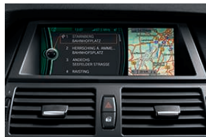
Navigation system features a high-resolution glare-free monitor and uses GPS satellites in conjunction with data stored on an internal hard drive. Includes 3-D daytime and nighttime maps, zoom, travel planner and an Assistance Window. The system provides Real Time Traffic Information on potential traffic problems and solutions. The hard drive offers 12 GB of space that can hold up to 2,000 of your favorite songs.
