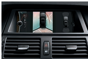
Rear-view Camera with Top View is automatically activated by shifting into reverse gear, or manually by pressing the Parking Assist button. The color display shows a real camera image that may include "static" and "track" lines to help you when backing up or parallel parking.
