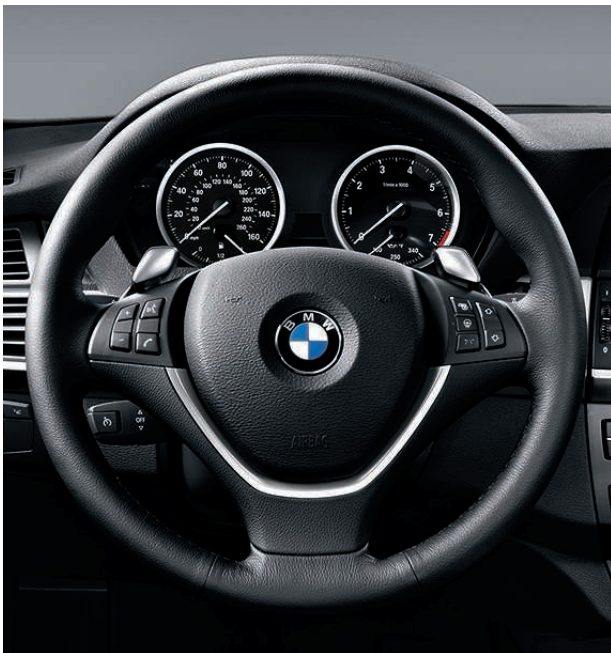
Three-spoke leather-wrapped multi-function sport steering wheel , featuring power tilt/telescoping adjustments, lets you keep both hands on the steering wheel while adjusting both the audio and a BMW-approved, Bluetooth® enabled mobile phone.
