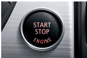
Engine Start/Stop button and remote key control the engine. First, insert the remote key into the starter switch slot. After the electronic identification system confirms that it is the correct remote, you can start (or later, turn off) the engine by pressing the Start/Stop button. (Foot must be on brake in order to start.)
