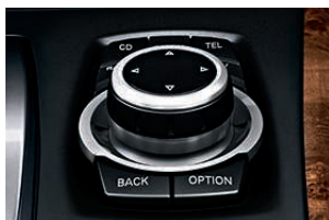
iDrive Controller , which is conveniently located on the center console, is the central command element for the iDrive system and can be rotated, pushed and tilted to operate various functions via the Control Display. Additionally, four frequently selected menus – CD, radio, Navigation system and telephone – can be called up using direct menu-control buttons.
