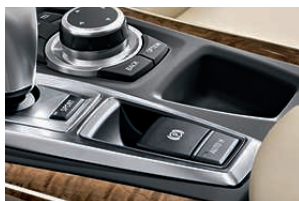
Electromechanical parking brake with Automatic Hold keeps the vehicle stationary whenever the vehicle comes to a stop, then releases the brake when the driver steps on the accelerator pedal.
