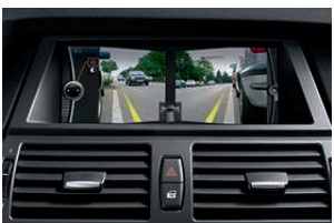
Side-view Cameras offer visual assistance when side visibility is limited, such as when exiting a parking garage or parking space. One camera is located on each front fender, just ahead of the wheel arches.
