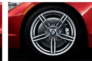
Double Spoke (Style 326M) light alloy wheels and run-flat performance tires. 1 In front: 19 x 8.0 wheels and 225/35 tires; in back: 19 x 9.0 wheels and 255/30 tires.
