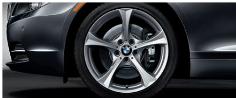
Star Spoke light alloy wheels (Style 276) , 18 x 8.0 front, 18 x 8.5 rear; and 225/40 front, 255/35 rear run-flat performance tires ¹ (Includes increased top-speed limiter).
