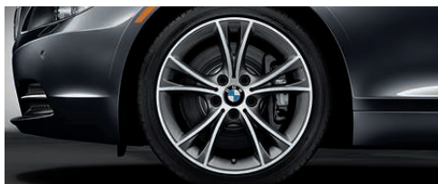
V Spoke light alloy wheels (Style 515) , 18 x 8.0 front, 18 x 8.5 rear; and 225/40 front, 255/35 rear run-flat performance tires ¹.
