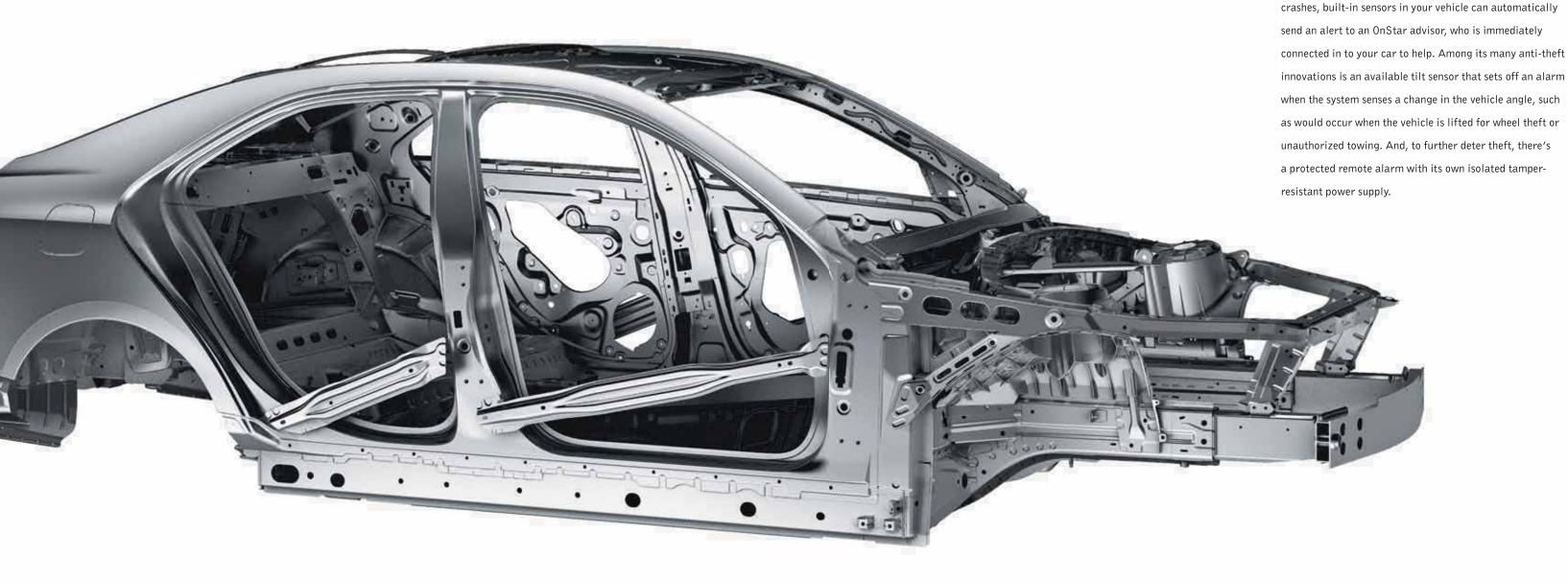
It starts with a protective safety cage constructed with ultra-high-strength steel alloys and other highly advanced materials for exceptional rigidity and strategically placed crumple zones. Then we add preventive safety features like the StabiliTrak Electronic Stability Control and full-function traction control systems. A sophisticated
