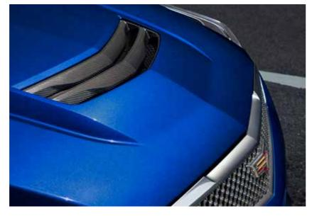
**V-tuned tech.** The V-Series is equipped with a carbon-fiber hood. The Carbon Fiber Package employs this lightweight yet incredibly strong material in the symmetrical design of a front splitter, hood vent and rear diffuser.
