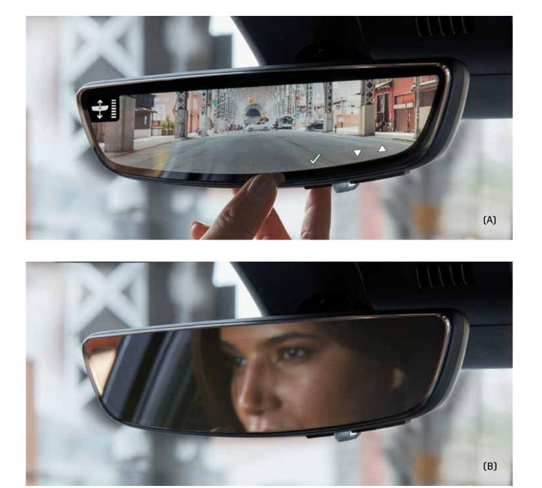
Top: Enhanced view with Rear Camera Mirror<sup>1</sup>(A). Bottom: Traditional reflection with rearview mirror (B). Facing page, left: The myCadillac mobile app.<sup>2</sup> Right: Streaming 4G LTE Wi-Fi.<sup>3</sup>
