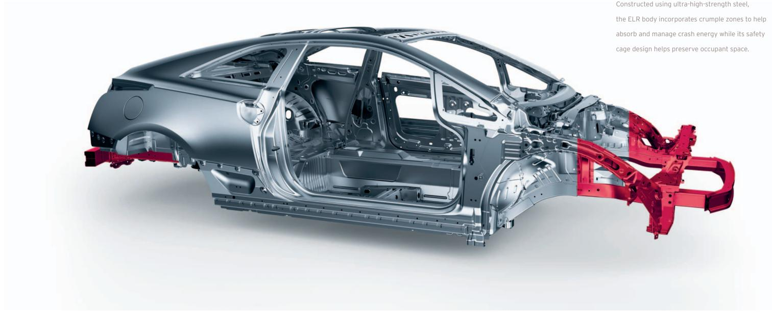
Constructed using ultra-high-strength steel,
