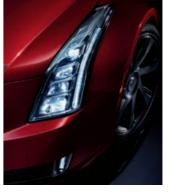
The signature, light-blade vertical headlamps combine classic styling with modern technology. Each contains four projector lenses powered by LEDs, individually precision-engineered for enhanced nighttime visibility as well as efficiency.
