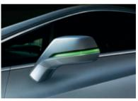
Lights on the side mirrors pulse green while the battery is charging and go dark when charging is complete.
