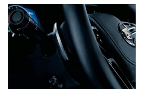
Dual-side paddle controls located behind the steering wheel provide regeneration on demand, putting energy back into your battery while simultaneously slowing you down. This technology is something you can only truly appreciate when you experience it from behind the wheel – especially in slow-and-go traffic where exclusive Regen on Demand<sup>™</sup> gives you the comfort of one-pedal driving.
