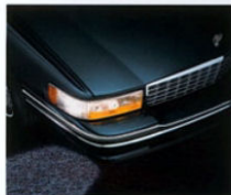
Cornering lamps, standard on all 1994 Cadillacs, illuminate the direction of your turn and add the power-ful, white, focused light from the headlamps.
