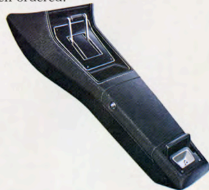
Floor Console. Mounts between front bucket seats. Contains storage compartment, ashtray for rear passengers and houses transmission shift lever when ordered.
