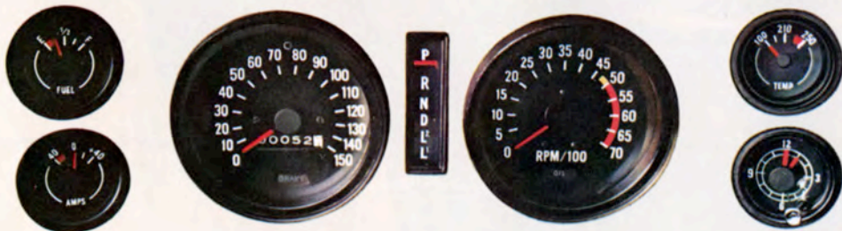
Special Instrumentation. Includes tachometer, ammeter, temperature gauge, electric clock.
