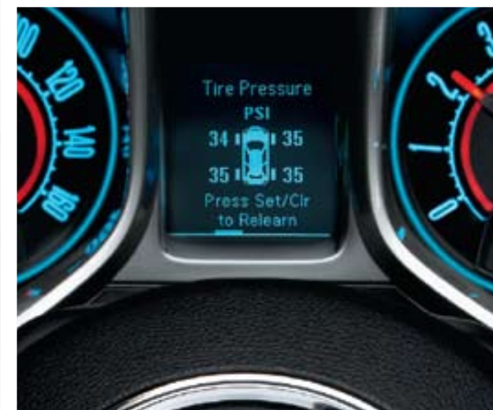
BOTTOM RIGHT: A TIRE PRESSURE MONITOR PROVIDES REAL-TIME READDUTS ON THE DRIVER INFORMATION CENTER.
