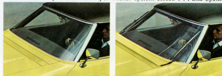
Hide-A-Way windshield wiper-washer system closed . . . and open.
