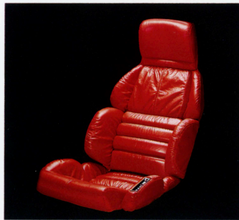
The optional leather sport seat includes power height and fore/aft adjuster, and power lumbar support feature.
