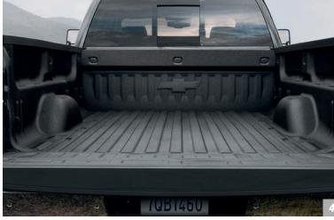
**1. GIVE THAT MAN A HAND.** Pocket hand grips built into the top of the side rails provide a boost into the bed.
