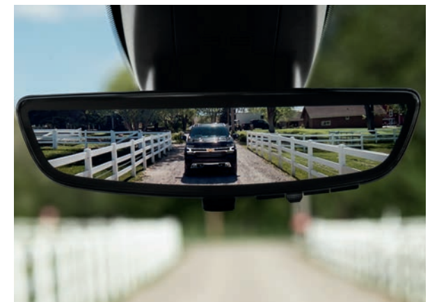
Rear Camera Mirror An available dual-function camera-based rearview mirror that provides a wider, less-obstructed field of view than a traditional rearview mirror.
