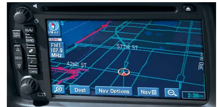
THE AVAILABLE INTEGRATED NAVIGATION RADIO 1 includes a full-color touch-screen display and the ability to play a CD or use the navigation DVD. Available in 3LT and SS models.
