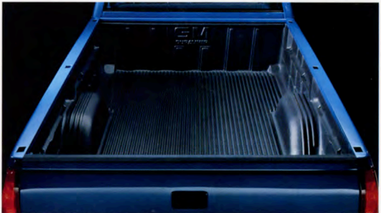
▲ A new-for-'91 optional bedliner (available with Fleetside models only) protects the C/K's cargo bed, sidewalls and inside tailgate panel from minor dents and dings during loading and unloading, and also provides additional insulation from road noise. See page 66 for additional information and warranty restrictions.
